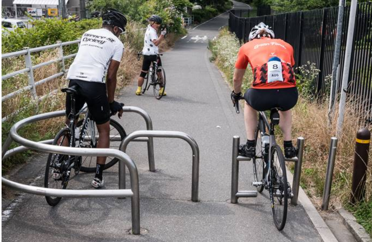
Example of a Single chicane and “cycle only” bollard
